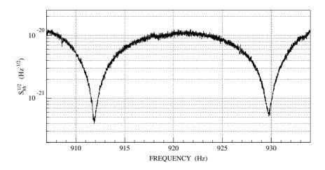
Figure 1. The strain noise power spectrum  $S_{hh}^{1/2}$  for the detector AURIGA (June 1997)
