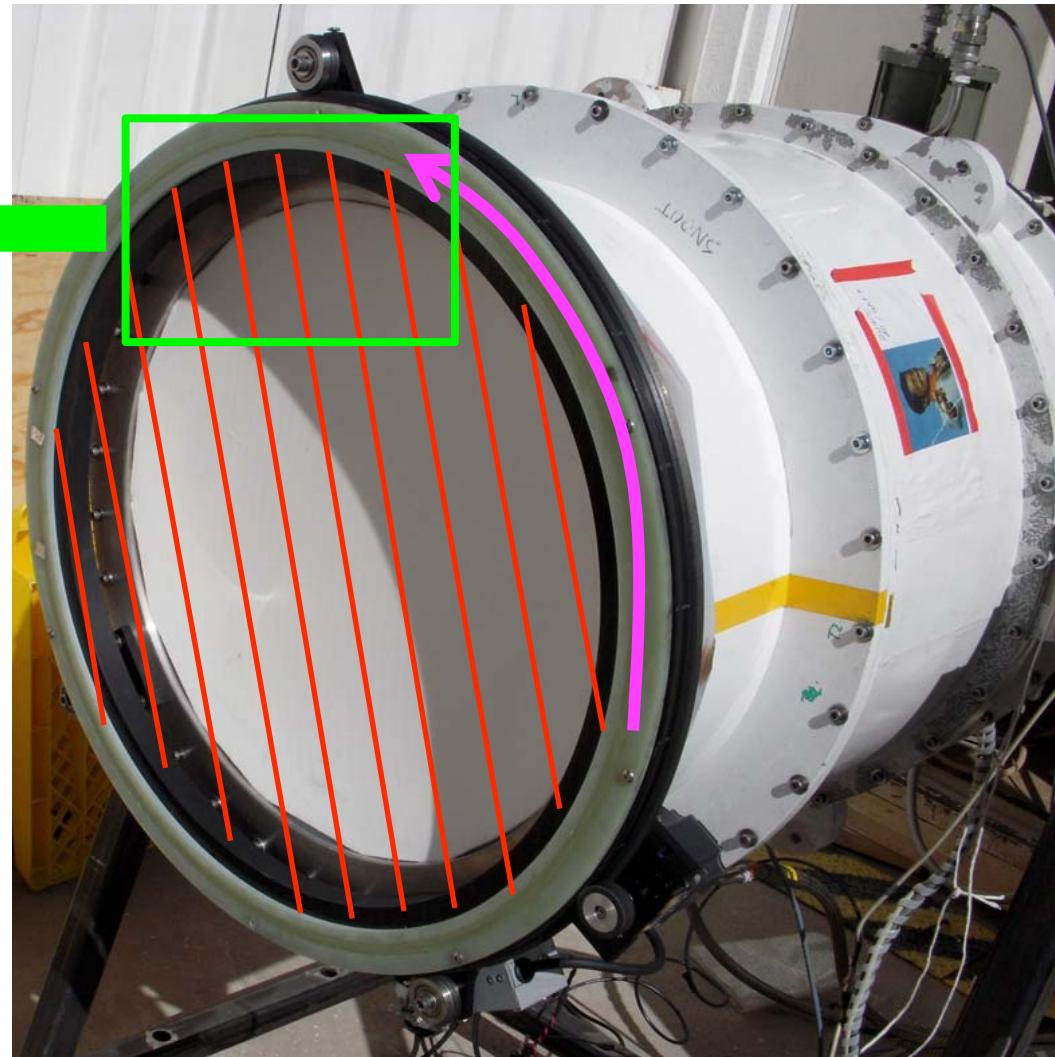
Polarized radiation ( $\approx 2K$ ) is created via the reflection of ambient temperature from the metal wire surface
