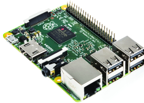
図 4.4: Raspberry Pi 2 model B
