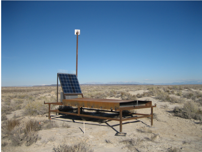
Figure 20: A SD in the field. There is a scintillator box under the roof to avoid the overheat caused by the sunshine. In a scintillator box, there are 2 layers of plastic scintillators. A SD electronics and a battery box are on the back of a solar panel. The height of an antenna pole is about 3m and the direction of the antenna is carefully adjusted for good communication with the communication tower.
