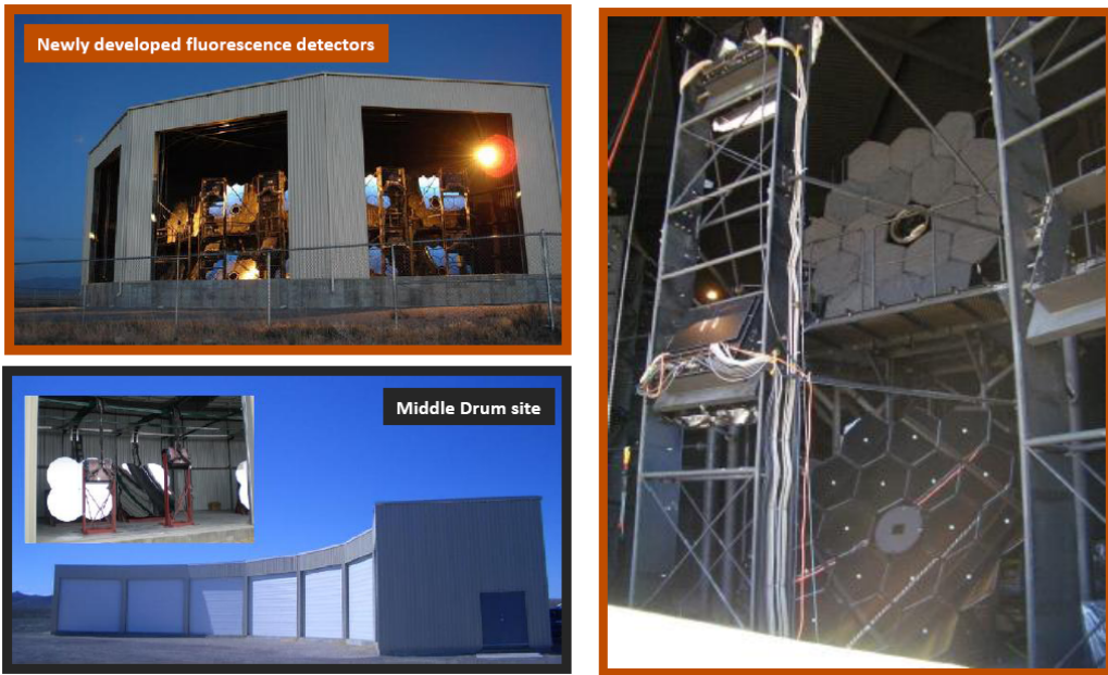
Figure 24: The BRM FD station (left top) and mirrors (right). The MD FD station and mirrors (left bottom).
