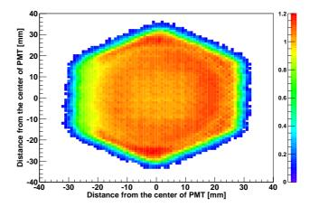
Figure 3.12: The typical non-uniformity map with 1 mm  $\times$  1 mm resolution of the photo-cathode of our photo-tube. It is normalized with the bins inside a circle with 36 mm diameter. The obtained map show an asymmetry long the x axis caused by the dynode structure of the PMT.
