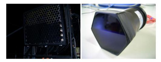
Figure 3.7: TA camera (left) and PMT of R9508 attached the UV filter (right).
