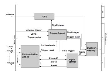
Figure 3.23: Block diagram of TA Central Trigger Distributor module.
