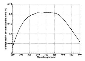
Figure 3.11: Multiplication values of the typical values of mirror reflectance, paraglas transmittance, UV filter transmittance and quantum efficiency of PMT.
