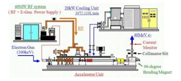
Figure 3.35: The schematic view of ELS system.
