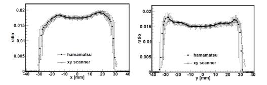
Figure 3.13: The comparison of results between the HAMAMATSU data and the data measured by XY-scanner. The left and right figure show the result along X axis and Y axis, respectively. The definition of the coordinate of x and y axis is the same as Fig. 3.12. Filled circle are the HAMAMATSU data and open circles are XY's scanners.
