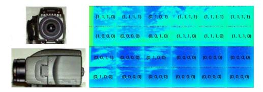
Figure 3.30: The overview of IR camera (left). The right figure is the 12 photographs taken by each telescope directions of FD. The number shows the analyzed cloud score on 4 horizontally categorized regions.
