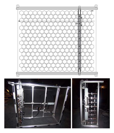
Figure 3.14: The schematic view and photograph of XY-scanner. The covering area of each LED is 2.5 PMTs vertically and 16 PMTs horizontally.
