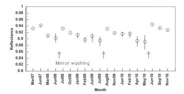
Figure 3.6: Variation in the mirror reflectance at 360 nm of a typical lower FD (FOV: 17.5-33 in elevation) of camera 04 at LR. The mirror was washed after these measurements in July 2007, August 2009 and May 2010 [53].
