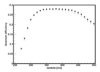
Figure 3.10: The typical quantum efficiency of photo-tubes. The data plot shows the median with one standard deviation error of all PMTs measured by HAMAMATSU PHOTONICS.
