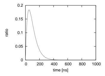
Figure 4.6: The response function of SDF. The time constant is 50 ns.
