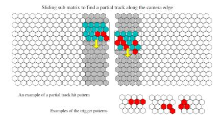
Figure 3.22: Schematic diagram of the partial track search near the boundary of a camera.
