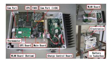
Figure 3.39: The electronics of TA SD.
