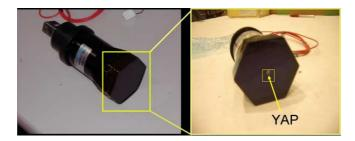
Figure 3.16: The UV pulsed light source located in front and center of the standard PMT, named YAP.
