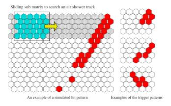
Figure 3.21: Schematic diagram of the track finding process.
