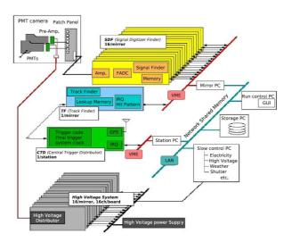
Figure 3.18: Block diagram of electronics and trigger system of the TA FD
