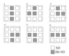
Figure 3.42: Trigger pattern taken at the TA surface array. If any three adjacent SDs have timing difference within 8  $\mu$ sec the trigger will be generated.
