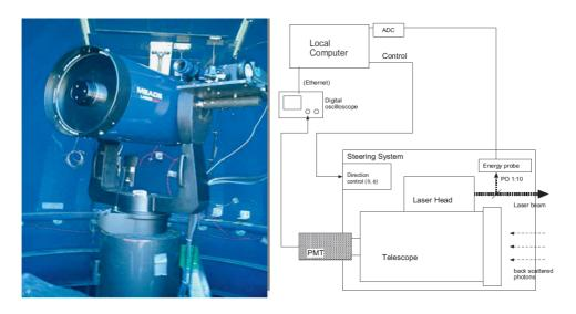
Figure 3.26: The overview of LIDAR system. A left picture is LIDAR's optical system (telescope, laser, etc), a right picture is a connection block diagram of device of LIDAR.
