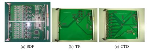
Figure 3.19: Photos of the trigger modules of TA fluorescence detector
