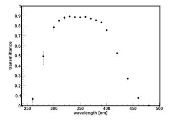
Figure 3.9: The typical transmittance of the UV filter in the front of phototubes. Data points are the medians for all the sampled filters with the bars corresponding the on standard deviation.
