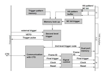
Figure 3.20: Block diagram of TA Track Finder module.
