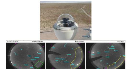
Figure 3.31: The photo of CCD fish-eye at LR station and picture taken at CLF, BRM and LR location. The yellow region shows the FOV of each FD, the green region shows the cover of CLF-LIDAR for online monitoring.
