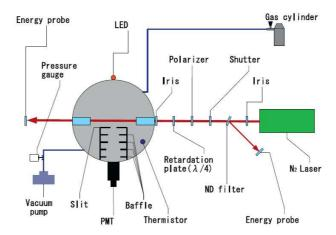
Figure 3.15: Measurement set up of CRAYS [75]
