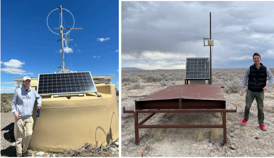
Figure 2.3: Left: Photo of the WCD used by Auger. Visible on top of the tank are the solar panel used for generating power and the scintillator and radio detectors installed as part of the recent AugerPrime upgrade [54]. Right: The scintillation detector used by TA. The scintillators and PMTs are housed underneath a 1.2 mm thick iron roof which shields the detector from the surrounding desert environment [24].
