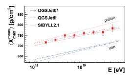
**Fig. 5.** The energy dependence of  $< X_{max} >$  for HiRes. The measured  $< X_{max} >$  is compared with the simulation (lines) with analysis biases included both for the measurement and simulation.
