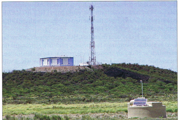
One of the 1660 surface-detector stations (foreground) and one of the four fluorescence-detector sites that make up the Pierre Auger Observatory in Argentina. Each surface-detector station contains 12,000 litres of water and is powered by a solar panel. Each of the fluorescence-detector sites houses six telescopes and a communications tower. (Image credit: Auger collaboration.)
