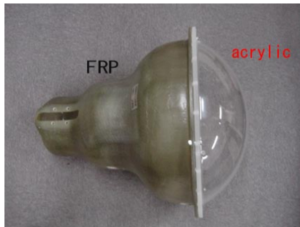
Figure 2.7: PMT case used to cover 20-inch PMT in the inner detector since SK-II period.
