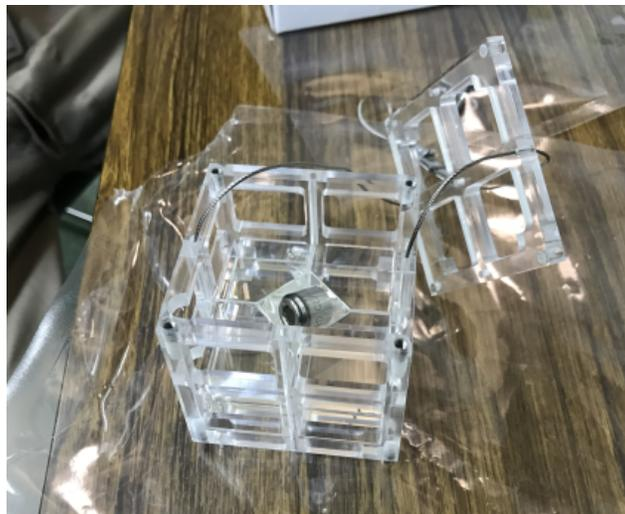
Figure 6.18: The Americium-Beryllium source and BGO crystal scintillator.
