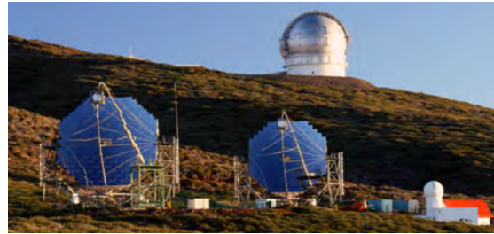
Fig. 9. MAGIC Stereo System with two Cherenkov telescopes of 17 m diameters, so far achieved the threshold energy of 25 GeV with the sum trigger. It locates near the mountain top of the Roque de los Muchachos on the Canary Island of La Palma. Two telescopes are located with the distance of 85 m.
