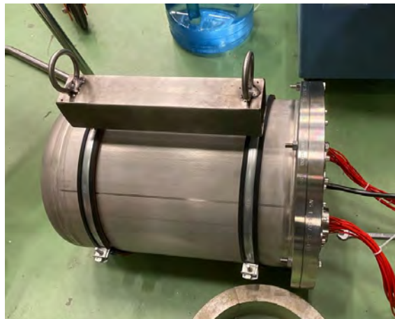
Fig. 41. Prototype of water-tight case for front-end electronics, that was designed to be 1 MPa tolerant under water.
