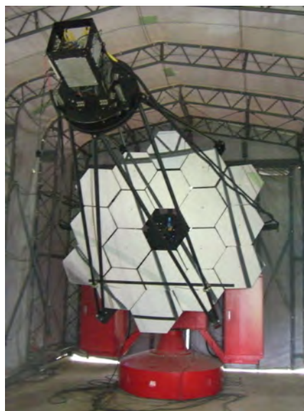
Fig. 13. Akeno atmospheric Cherenkov telescope of 3 m diameter, located in the Akeno Observatory.
