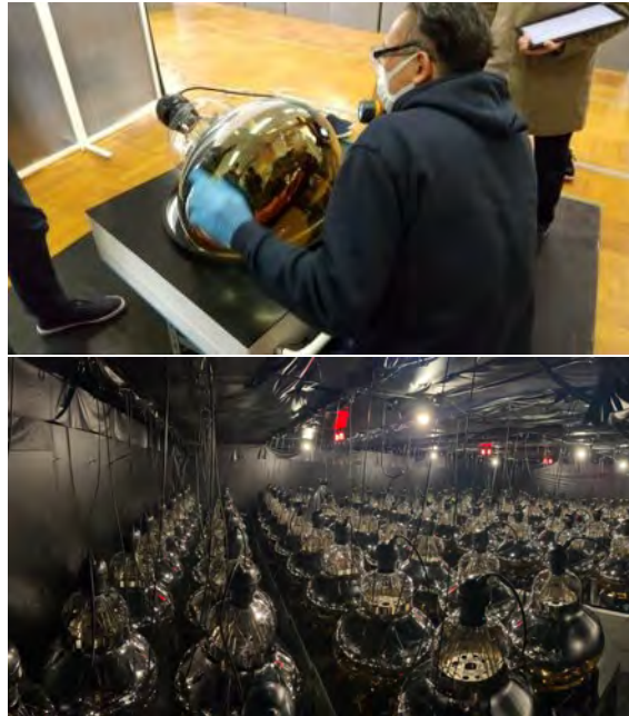
Fig. 40. Visual inspections of PMTs (top). Dark room for long term stability check of 100 PMTs (bottom).
