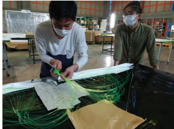
Fig. 10. A surface detector for the TALE-infill array that was being assembled at the Akeno Observatory. The student was aligning the ends of bundled fibers.
