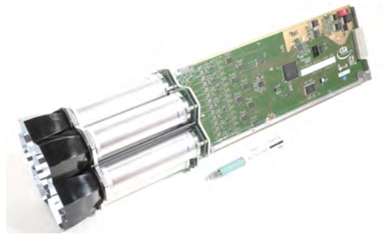
Fig. 3. Camera cluster for the Large Size Telescope (LST) developed by CTA-Japan. This cluster consists of seven high quantum efficiency photomultipliers (R11920-100), CW High Voltages, pre-amplifier, Slow Control Board, DRS4 Ultra fast waveform recording system and Trigger. The LST camera can be assembled with 265 of these clusters, cooling plates and camera housing.
