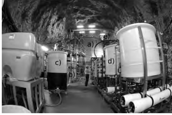
Fig. 15. In the LAB-E cavern, the 200-ton tank (a) with currently 240 photo-multipliers installed, the Gd pre-mixing and pre-treatment 15-ton tank (b), the selective filtration system (d), Gd removal resins (c) for test and a device to measure the water transparency (e) have been installed.
