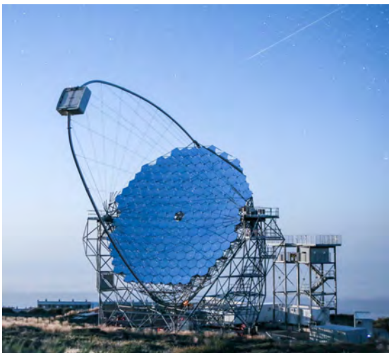
Fig. 5. The Large Size Telescope prototype (LST-1) constructed at Observatorio de Roque de los Muchachos is now in the engineering run. The diameter of dish and mirror surface area are 23 m and 400 m 2 .
