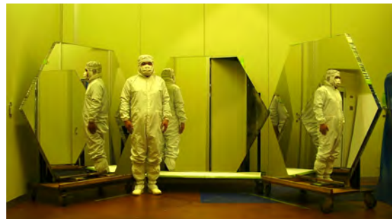
Fig. 4. The high precision segmented mirrors for the Large Size Telescope (LST) developed by CTA-Japan in cooperation with Sanko Co.LTD. The mirror is made of a 60-mm thick aluminum honeycomb sandwiched by 3-mm thin glass on both sides. A surface protection coat consisting of the materials \text{SiO}_2 and \text{HfO}_2 is applied to enhance the reflectivity and to elongate the lifetime.
