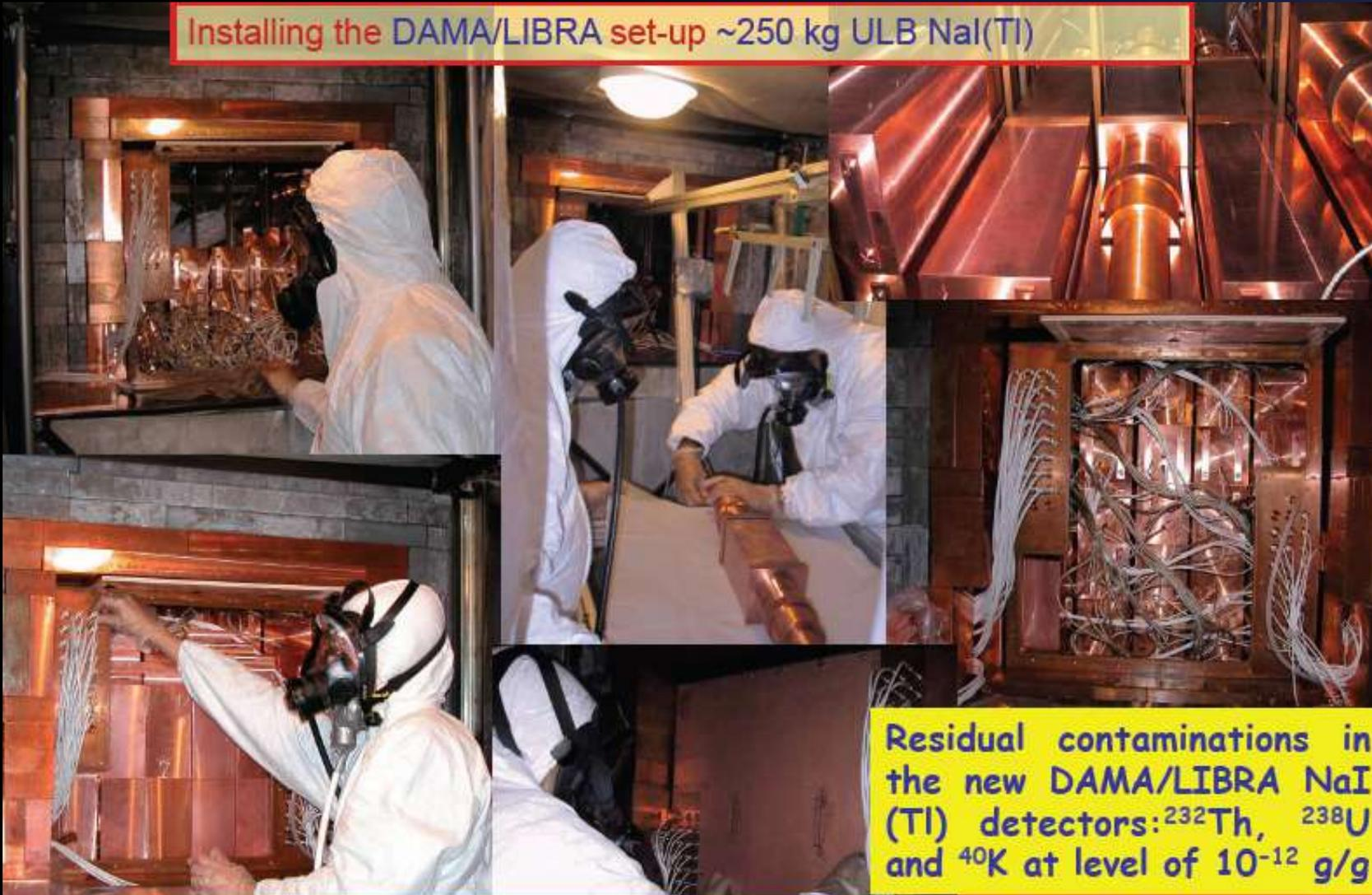
Residual contaminations in the new DAMA/LIBRA NaI (Tl) detectors:  $^{232}\text{Th}$ ,  $^{238}\text{U}$  and  $^{40}\text{K}$  at level of  $10^{-12}$  g/g
