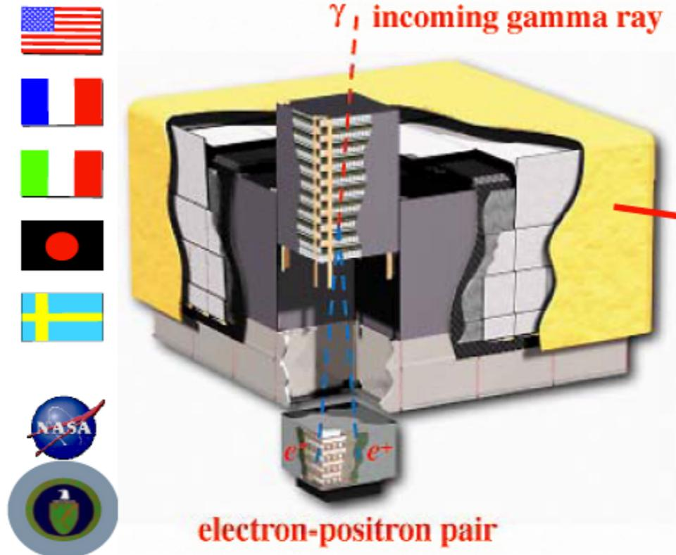
$\gamma$ -ray converts in LAT to an electron and a positron ; tracking these give us the direction and energy of the photon.
