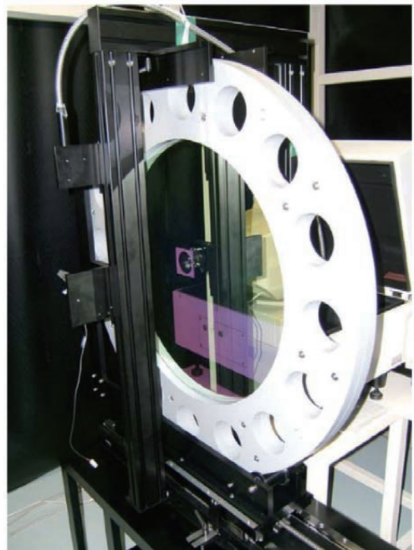
図6 開発中のすばる HSC 用狭帯域フィルター (Materion [旧 Barr Associates] 社と協力)。 Subaru/HSC narrow band filter under development (collaboration with Barr Associates Inc.)
