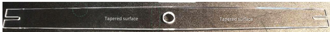
Fig.3: The prototype blade. Notice that the two heels at the center, in this version are not present. The two blockets that constitute the heels, meant to optimize the Q, have been constructed too, but they will be attached to the blade by means of HCB (Perugia).
