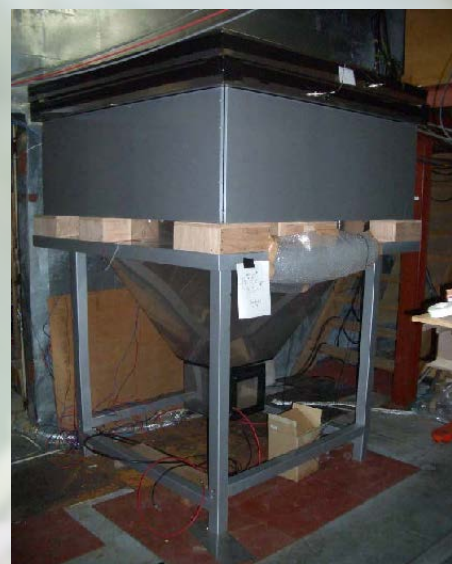
Fig. 3. 0.5-m 2 plastic scintillation counter for a new neutron telescope.
