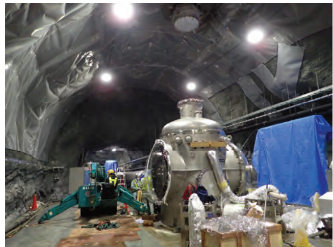
Fig. 5. Cryostat for the cryogenic mirror and the shaft for the vibration isolation system.
