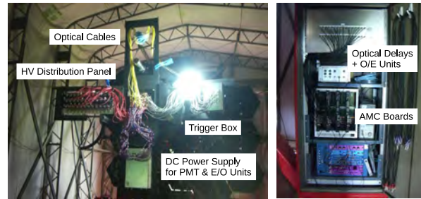
Fig. 6. R & D system of 32 pixel imaging camera and electronics installed to the Akeno atmospheric Cherenkov telescope.
