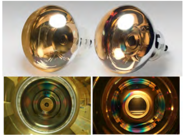
Fig. 38. Photographs of two new photo-sensors. The top left image shows a Hybrid Photo-Detector and the top right picture shows a Box and Line PMT. The electrodes for signal amplification of each sensor are in the bottom panel.
