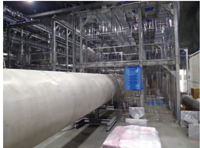
Fig. 10. Chamber and beam tube for the input mode cleaner.
