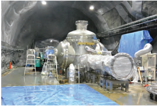
Fig. 16. KAGRA cryostat at center room of KAGRA site. The cryocoolers and cryo duct are connected to the cryostat.
