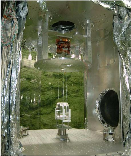
Fig. 11. A sapphire mirror and cryogenic suspension system
