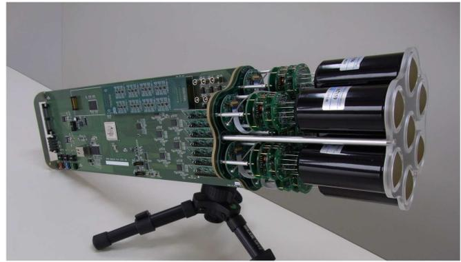
Fig. 4. Camera cluster for the Large Size Telescope (LST) developed by CTA-Japan. This cluster consists of seven high quantum efficiency photomultipliers (R11920-100), CW High Voltages, pre-amplifier, Slow Control Board, DRS4 Ultra fast waveform recording system and Trigger. The LST camera can be assembled with 400 of these clusters, cooling plates and camera housing.
