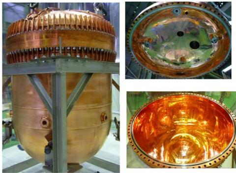
Fig. 3. Photo of IVC (left). The inner surface of upper part (right, top) and lower part (right, bottom).
