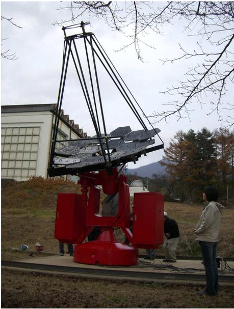
Fig. 6. 3 m Cherenkov telescope installed at the Akeno observatory as a test bench for future ground-based gamma-ray observatories.
