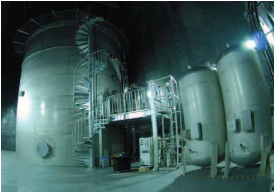
Fig. 3. A water tank (left side) for shielding from gamma ray and neutrons. The liquid xenon detector will be located at the center of the tank.
