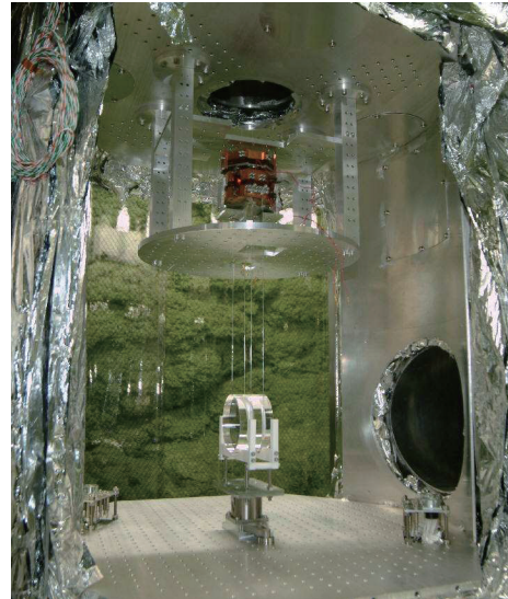
Fig. 5. a sapphire mirror and cryogenic suspension system.
