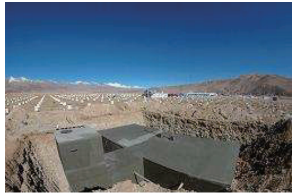
Fig. 10. Prototype muon detector viewed from outside, just before being covered with soil.
