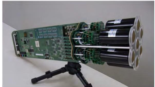
Fig. 3. Camera cluster for the Large Size Telescope (LST) developed by CTA-Japan. This cluster consists of seven high quantum efficiency photomultipliers (R11920-100), CW High Voltages, pre-amplifier, Slow Control Board, DRS4 Ultra fast waveform recording system and Trigger. The LST camera can be assembled with 265 of these clusters, cooling plates and camera housing.
