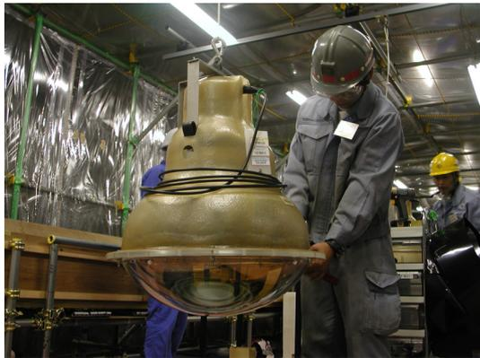
Fig. 1. PMTs are assembled with acrylic and FRP cases to prevent shock wave production.
