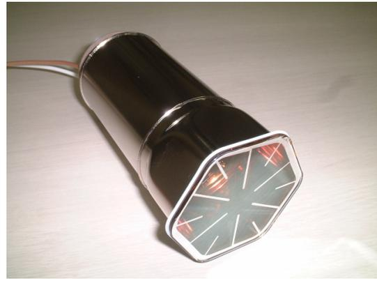
Fig. 4. Hexagonal PMT for the 800 kg detector.
