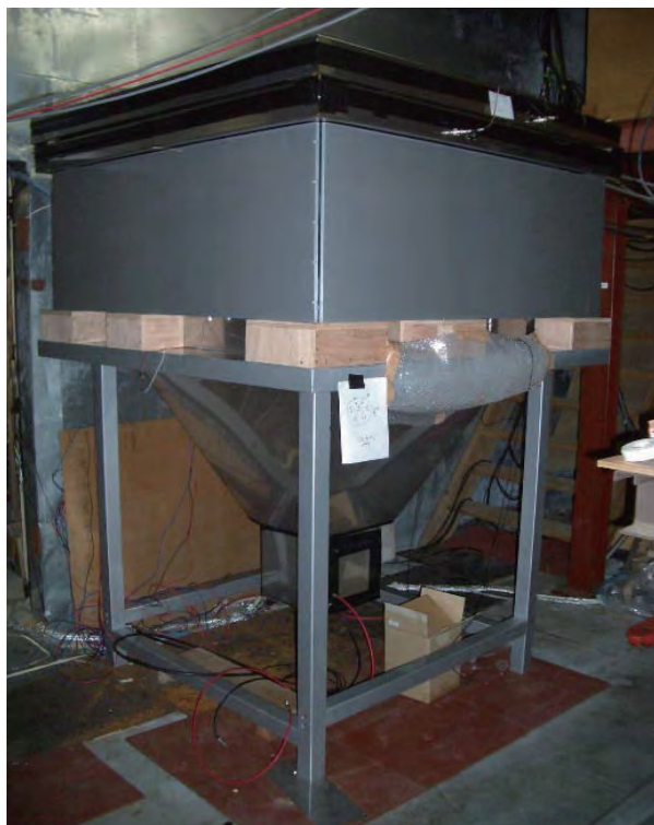
Fig. 3. 0.5-m 2 plastic scintillation counter for a new neutron telescope.
