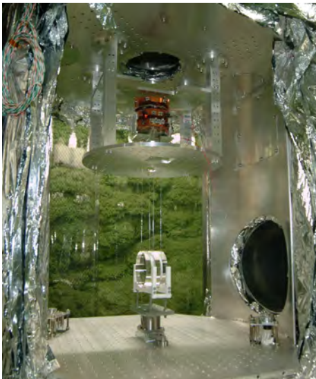
Fig. 11. A sapphire mirror and cryogenic suspension system
