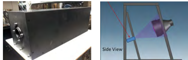
Fig. 39. LED flusher (left) and the schematic view of the installation on LC (right).
