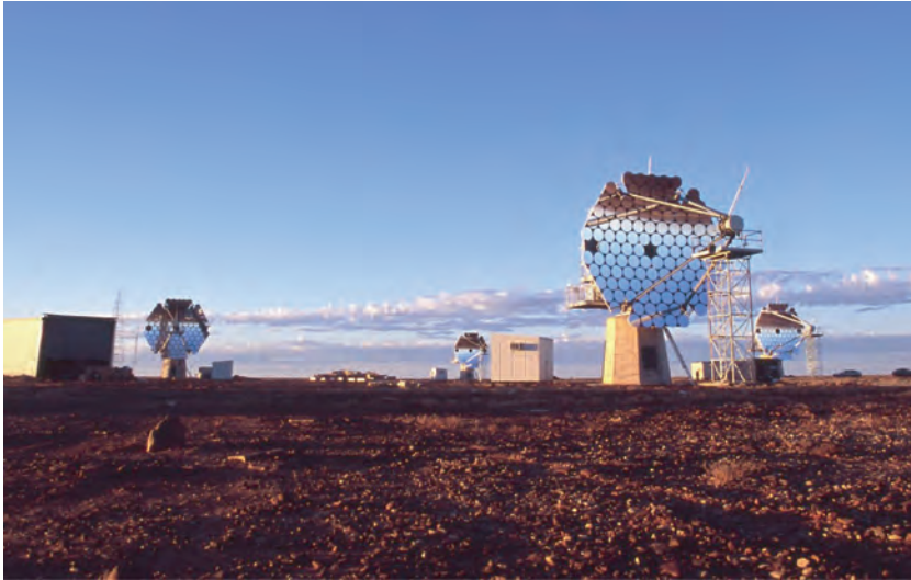
The system of four imaging atmospheric Cherenkov telescopes of 10m diameter of CANGAROO project for detection of very high energy gamma-rays. The whole system is in operation since March 2004 in Woomera, South Australia.
