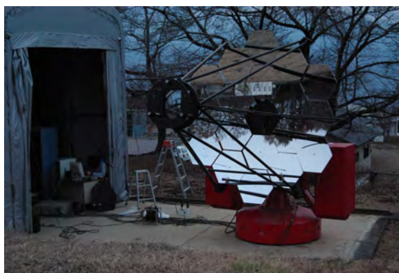
Fig. 6. Akeno atmospheric Cherenkov telescope with 18 segment mirrors readjusted as the Davies-Cotton optics.
