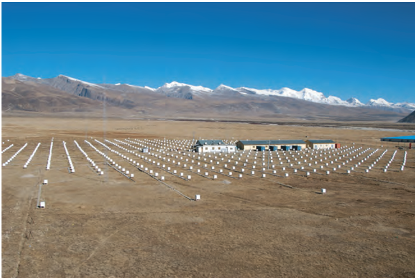
Tibet-III air shower array (37000 m 2 ) at Yangbajing, Tibet (4300 m in altitude).
