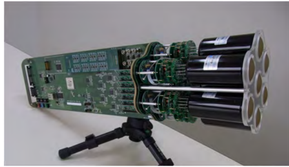
Fig. 3. Camera cluster for the Large Size Telescope (LST) developed by CTA-Japan. This cluster consists of seven high quantum efficiency photomultipliers (R11920-100), CW High Voltages, pre-amplifier, Slow Control Board, DRS4 Ultra fast waveform recording system and Trigger. The LST camera can be assembled with 400 of these clusters, cooling plates and camera housing.
