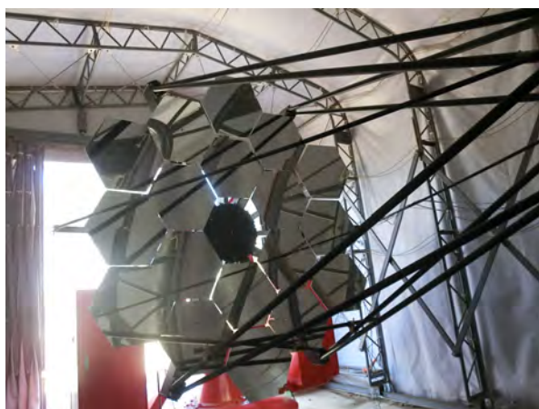
Fig. 5. Akeno atmospheric Cherenkov telescope with 18 segment mirrors recoated and assembled back to the structure.
