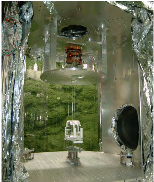
Fig. 15. A sapphire mirror and cryogenic suspension system
