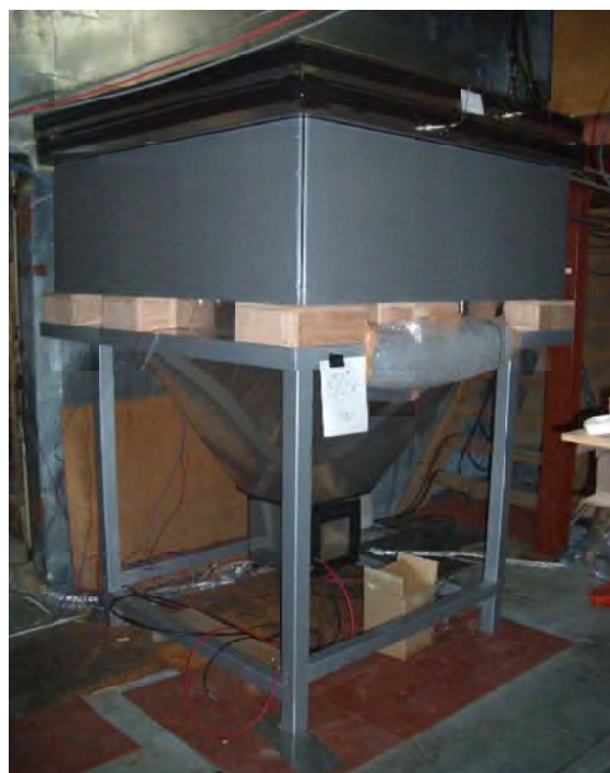
Fig. 3. 0.5\text{-m}^2 plastic scintillation counter for a new neutron telescope.
