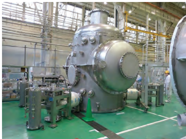
Fig. 9. Assembled KAGRA cryostat in Toshiba Keihin Product Operations
