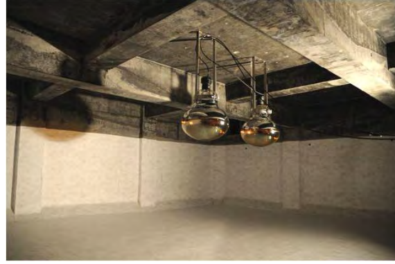
Fig. 23. PMTs mounted on a MD cell.
