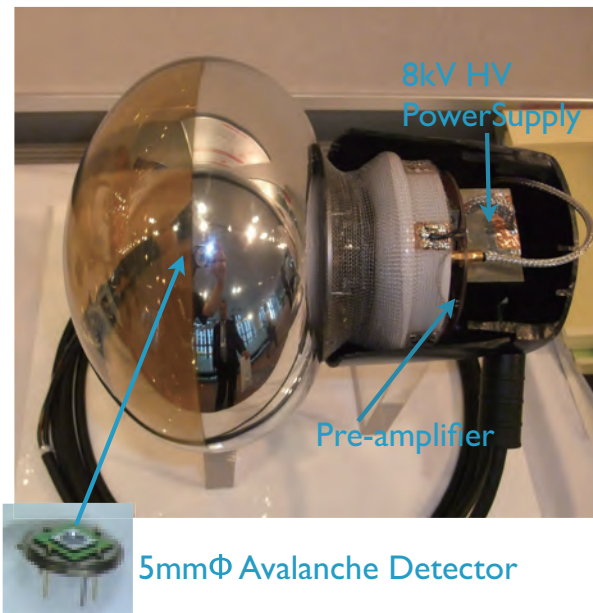
Fig. 33. 8-inch hybrid photo detector prototype.
