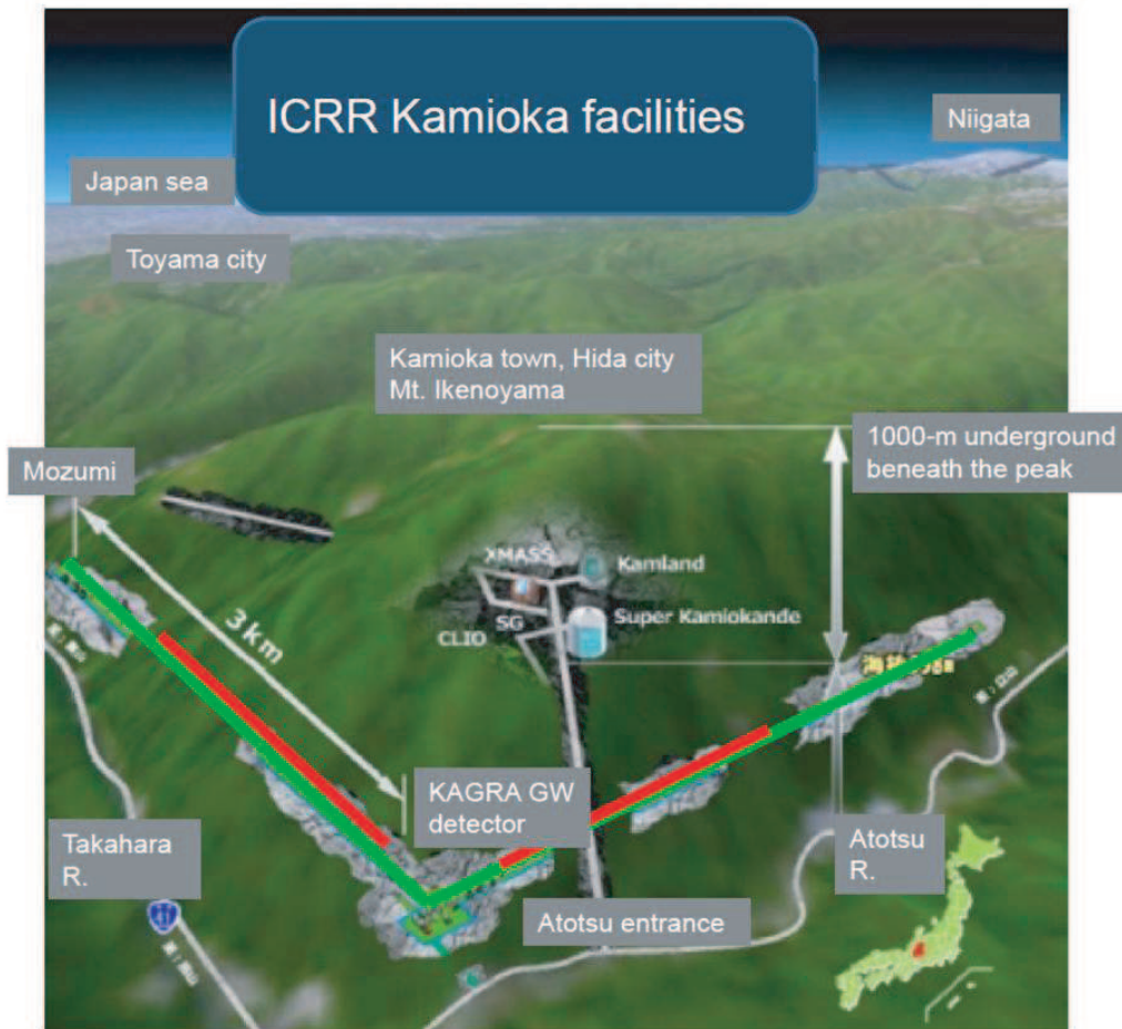
Fig. 20. An overall view of KAGRA. Red lines indicate baselines of GIF.
