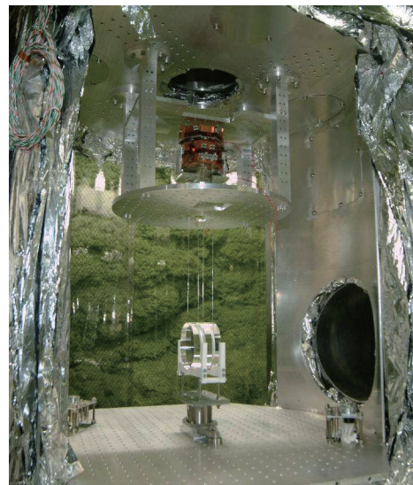
Fig. 8. a sapphire mirror and cryogenic suspension system.
