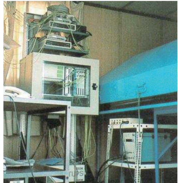
Fig. 2. AGASA scintillation detector and data acquisition system.
