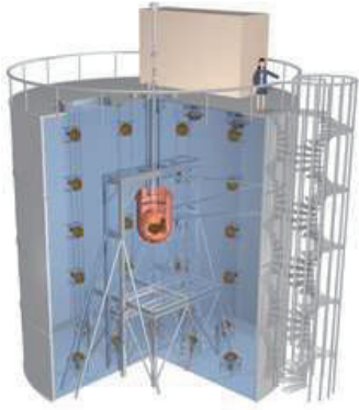
Fig. 3. Schematic view of the water tank and the liquid xenon vessel.
