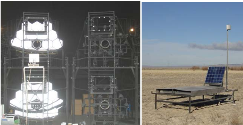
Air fluorescence telescopes (left) and a scintillator surface detector (right) of the Telescope Array experiment under construction in Utah, USA for the study of extremely high energy cosmic rays.
