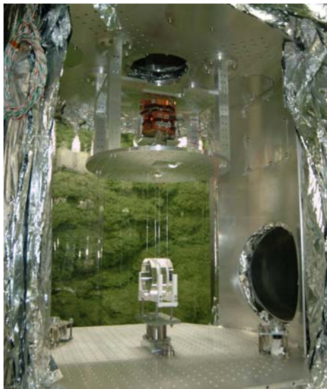
Fig. 5. a sapphire mirror and cryogenic suspension system.
