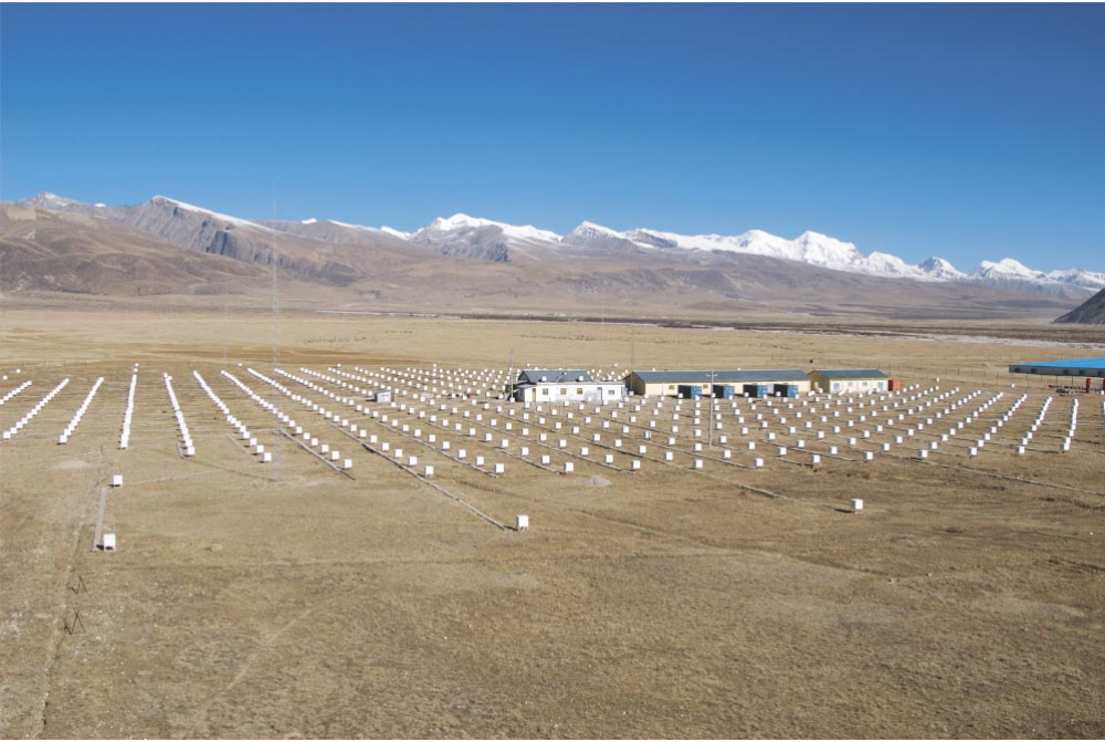
Fig. 4. Tibet-III air shower array (37000 m 2 ) at Yangbajing, Tibet (4300 m in altitude).
