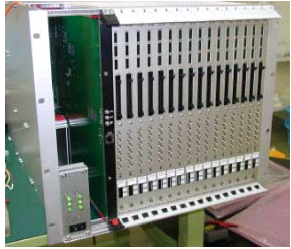
Fig. 6. Test setup of readout and trigger for the fluorescence telescope.
