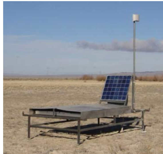
Fig. 8. A scintillator ground detector deployed in the field.
