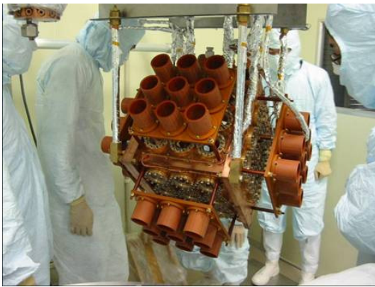
Fig. 2. 3 kg fiducial volume liquid xenon detector constructed for R&D study
