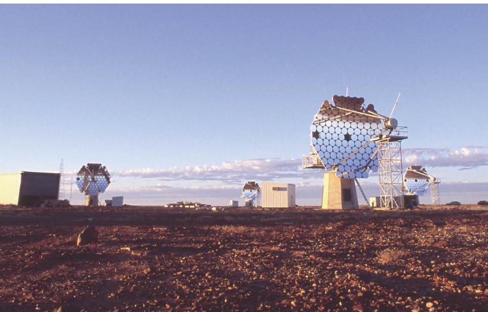
Fig. 3. The system of four imaging atmospheric Cherenkov telescopes of 10 m diameter of CANGAROO project for detection of very high energy gamma-rays. The whole system is in operation since March 2004 in Woomera, South Australia..
