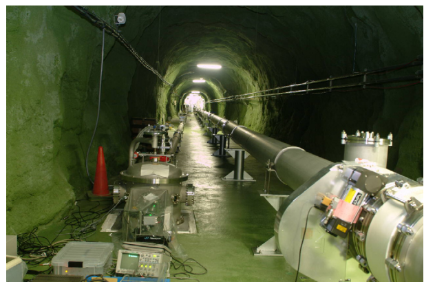
Fig. 3. 100 m baseline laser interferometers for gravitational wave and geophysics in Kamioka mine.
