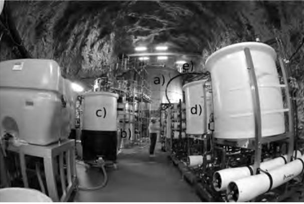
Fig. 17. In the new cavern, the 200-ton tank (a) with currently 240 photomultipliers installed, the Gd pre-mixing and pre-treatment 15-ton tank (b), the selective filtration system (d), Gd removal resins (c) for test and a device to measure the water transparency (e) have been installed.
