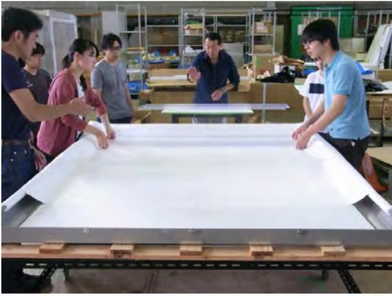
Fig. 22. Assembly of a plastic scintillator counter at the assembly hall of the Akeno Observatory
