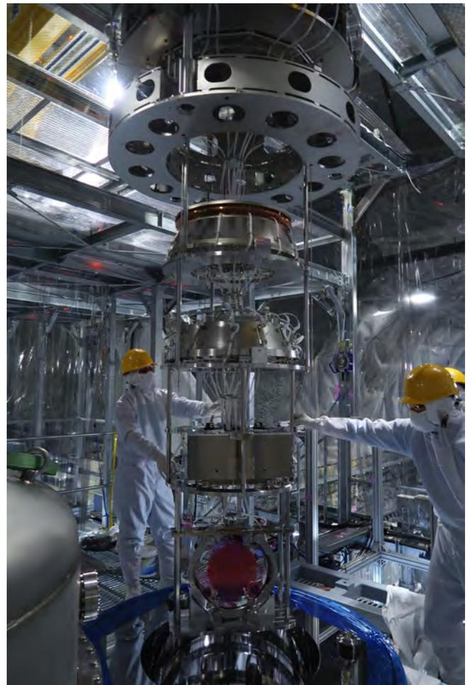
Fig. 4. Type-B vibration isolation system for beam splitter.
