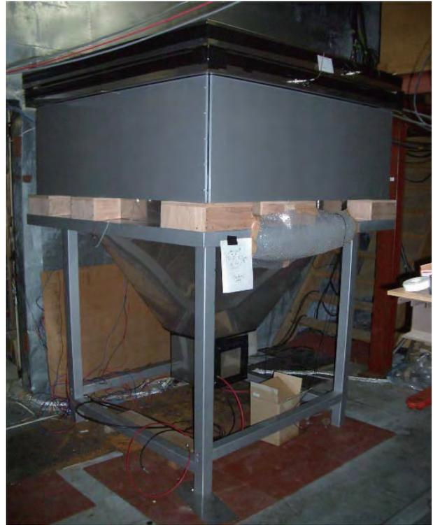
Fig. 3. 0.5-m<sup>2</sup> plastic scintillation counter for a new neutron telescope.
