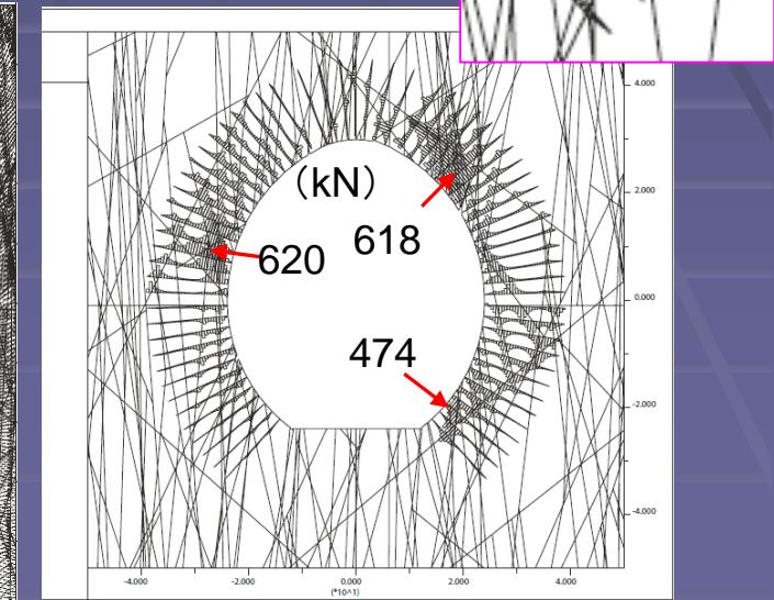
Displacement of Right and Left Side Wall are nearly same because of Symmetrical Joint Dip Angle ( $\pm 70 \sim 90^\circ$  ).
