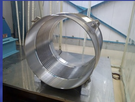
Bellows for each duct
