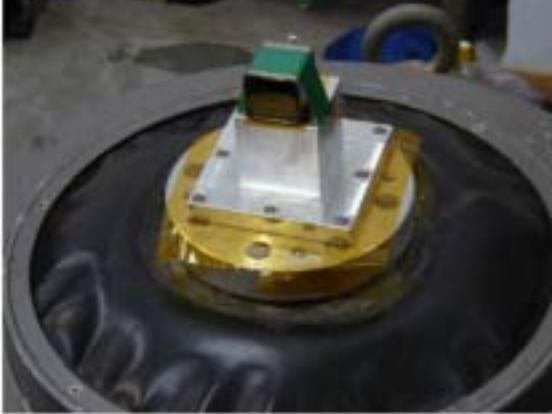
Fig. 9. MAPMT R8900-M25 attached to the vibration genera
