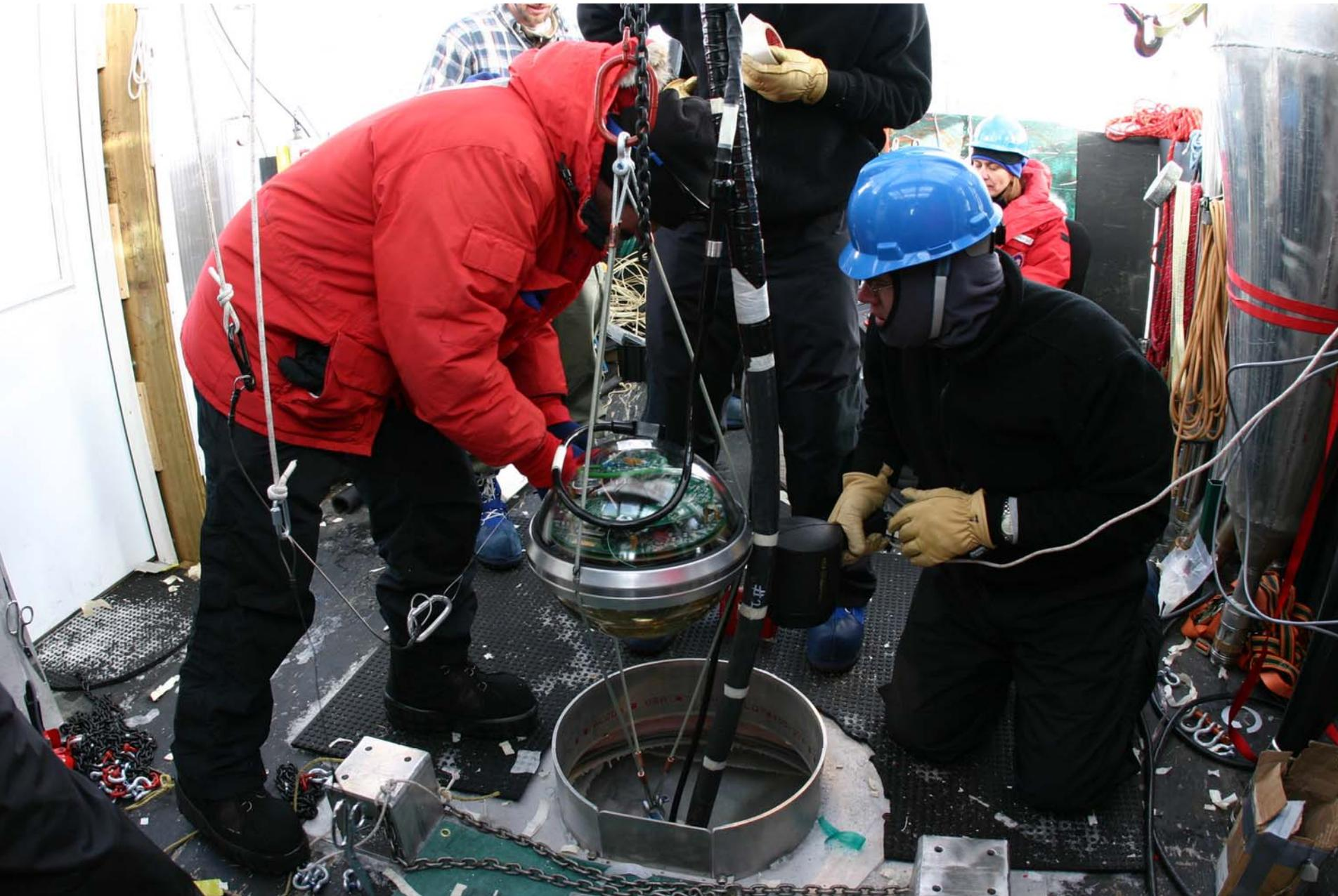
IceCube string anchored between IceTop tanks
