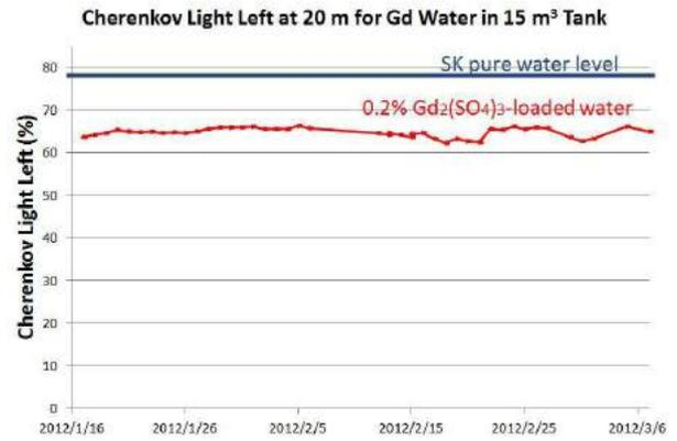
Fig. 24. Time variation of the estimated light yield during the Gd-loaded water circulation run. 0.2% Gd<sub>2</sub>(SO<sub>4</sub>)<sub>3</sub>-loaded water was circulated through the selective filtration system. The vertical axis shows Cherenkov light yield at a distance of 20 meters estimated from the measured water transparency at each wavelength.
