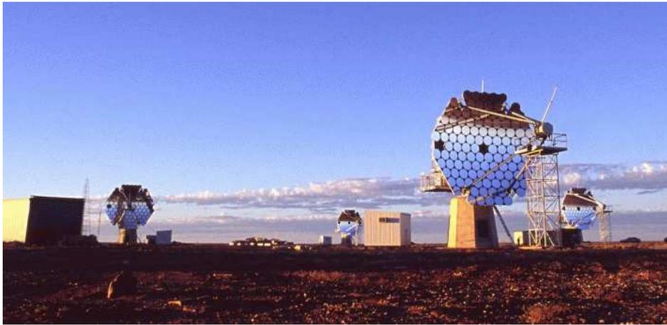
Fig. 1. The CANGAROO-III telescope system consisting of four 10 m imaging atmospheric Cherenkov telescopes located near Woomera, South Australia. They are called 'T2', 'T4', 'T3', and 'T1' from the left and are set at the corners of a diamond of 100 m sides.
