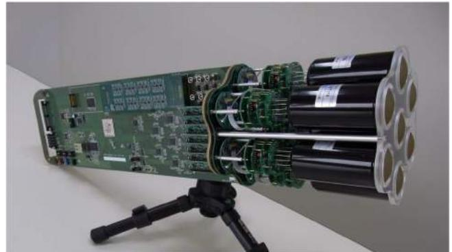
Fig. 9. PMT Cluster consists of seven photomultipliers, CW-HVs, Preamplifiers, readout electronics, and trigger system. Signals are digitized in this module and sent to DAQ camera server system via Ethernet.
