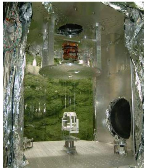
Fig. 3. A sapphire mirror and cryogenic suspension system
