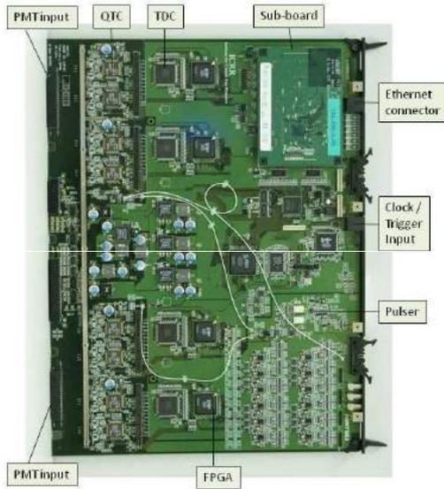
Fig. 20. New front-end electronics, QBEE. PMT signals are fed through the backplane (left side). The Ethernet cable for the data readout and the board control is connected at the front panel (right side) as well as the UTP cable for the 60MHz system clock input.
