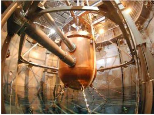
Fig. 3. Detector with copper vessel and an inner view of the water shield
