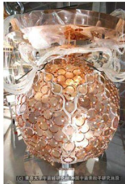
Fig. 2. PMT holders and backside of PMTs
