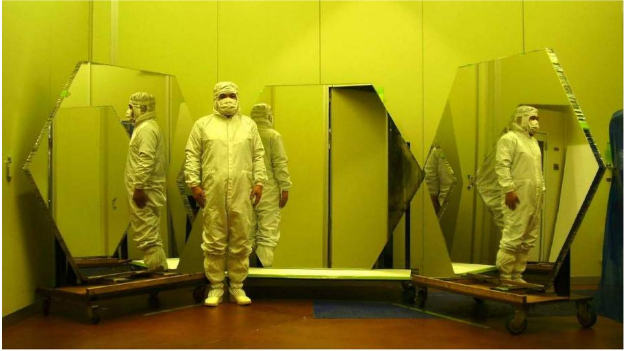
Fig. 5. Hexagonal shape mirrors of 1510mm size prototyped by Sanko LTD. The area is about  $2\text{m}^2$  and the focal length is 28m. Mirrors are produced with the cold slump technique. The mirror surface is protected with the multi-layer coating with  $\text{SiO}_2$  and  $\text{HfO}_2$  which are produced by sputtering method.
