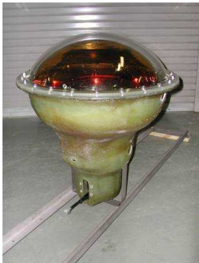
All PMTs were packed in acrylic and FRP cases to prevent shock-wave.
