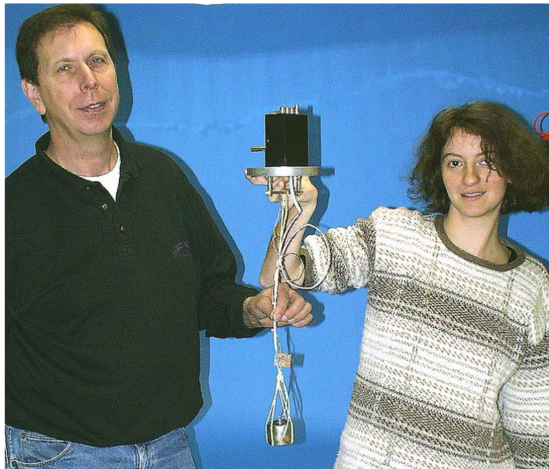
A first "bare" HPGe detector
