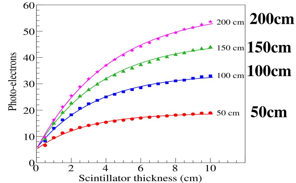
FIG. 6. Mean photo-electrons as function of thickness for  $\lambda = 50, 100, 150, 200$  cm. Data fitted by  $PE = a - b \times e^{(-x/c)}$ . Y-axis intercept  $a - b = (5.2 \pm 0.5)$  and  $c = (3.6 \pm 0.5)$  cm.
