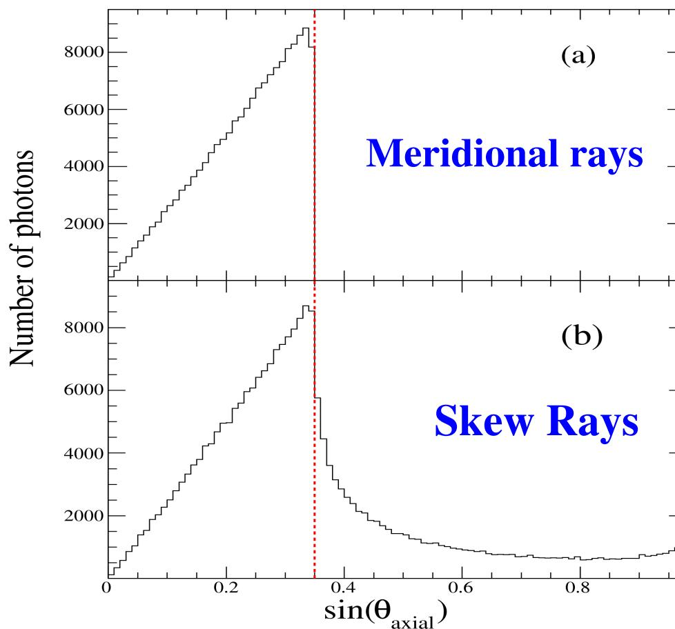
Trapping Efficiency of meridional rays = 3.2 %
