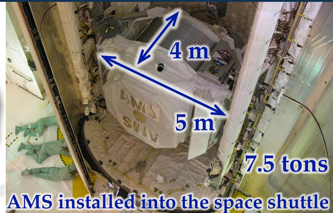
AMS installed into the space shuttle
