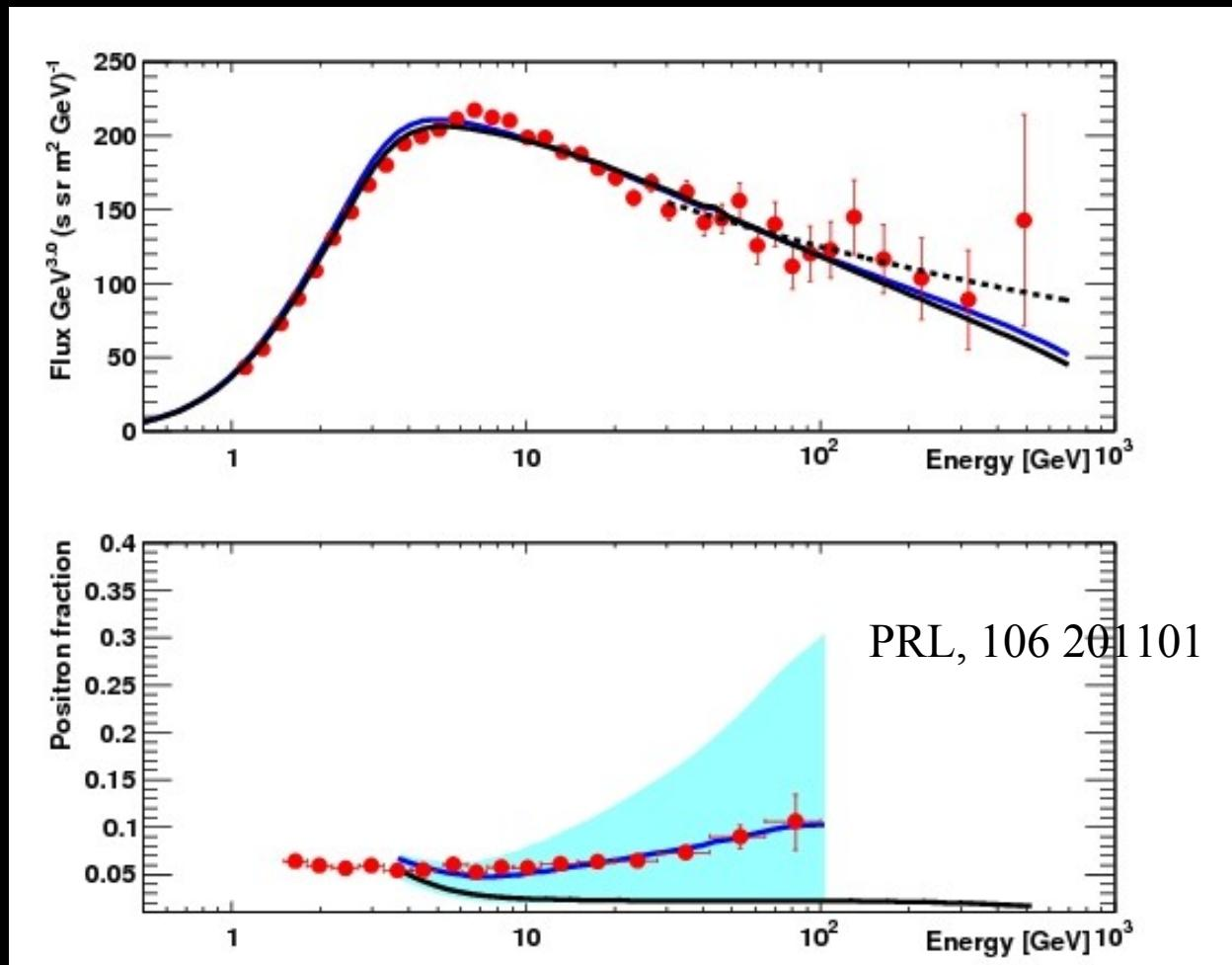
Solid line GALPROP calculation for a diffusion reacceleration model; the dotted line is a single power-law fit to the data above 30 GeV; the dashed-dotted line is a GALPROP calculation including a component from additional cosmic-ray electron sources.
