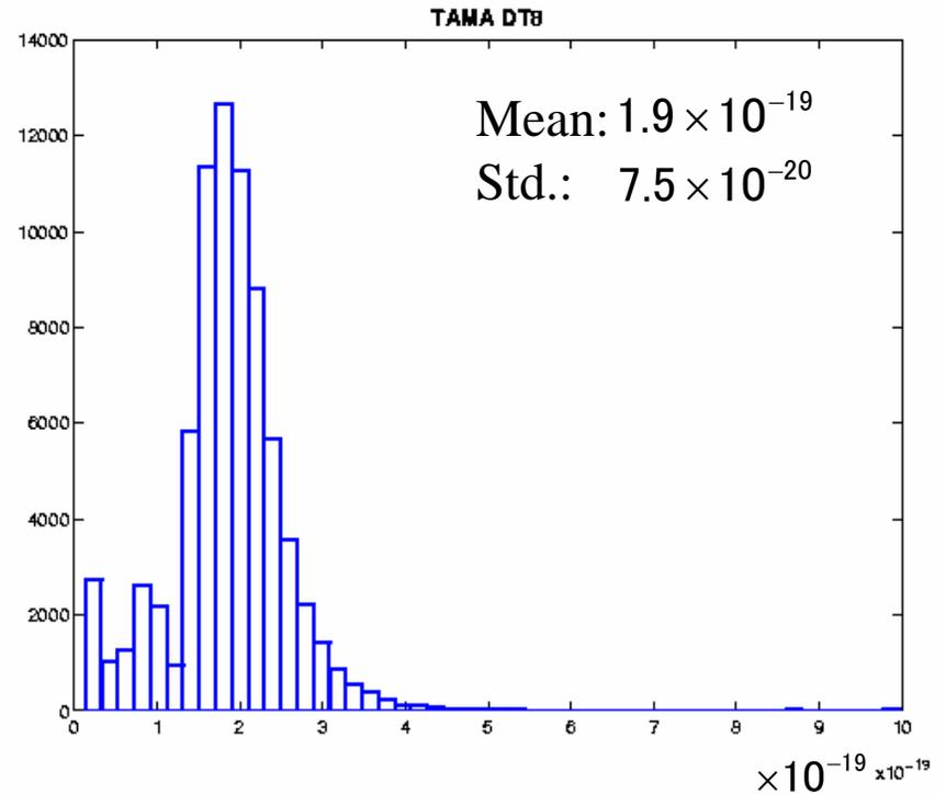
The fluctuation of noise power in DT8 is small.
