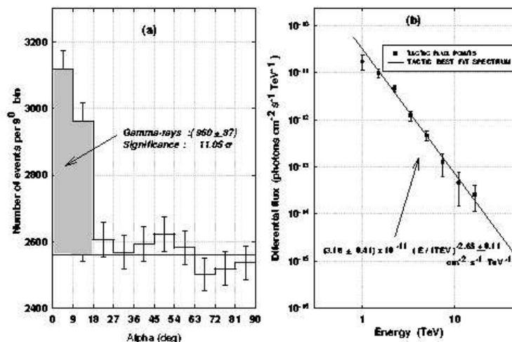
**Figure 5.** (a)  $\gamma$ -ray Signal and (b) Energy spectrum of CRAB nebula from TACTIC at Mt Abu
