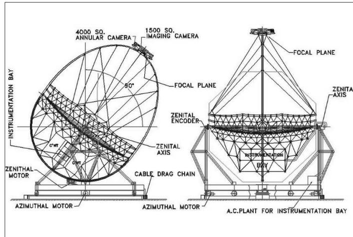
**Figure 9.** A schematic of the MACE  $\gamma$ -ray telescope planned to be set up at Hanle
