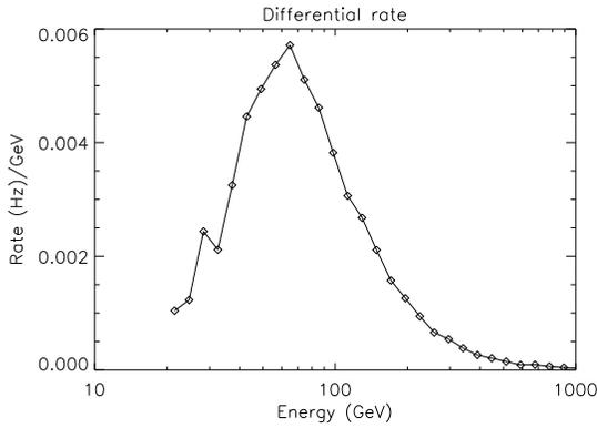
**Figure 7.** Expected differential  $\gamma$ -ray count rate spectrum from Crab nebula.
