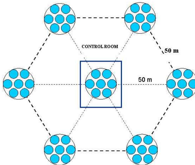
**Figure 6.** Layout of 7 telescope HAGAR array
