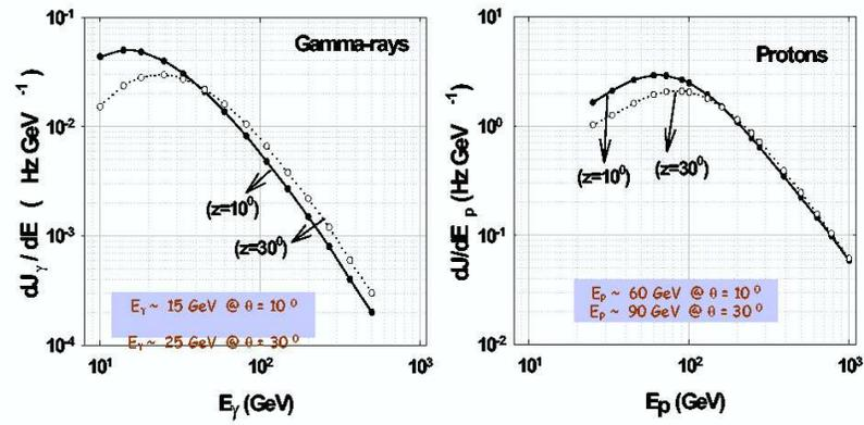
**Figure 10.** Differential detection rate of events as a function of the primary energy. The left panel is for  $\gamma$ -ray and right panel for proton primaries.
