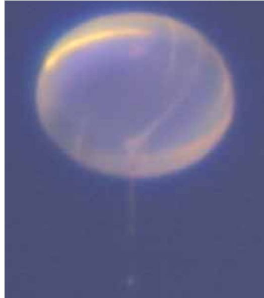
Figure 11. Photograph of the inflated 0.17 MCM balloon at 30 km (~100,000 ft) float altitude
