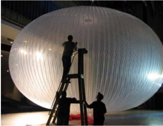
Figure 10. Photograph of the inflated scale model of the 0.17 MCM
