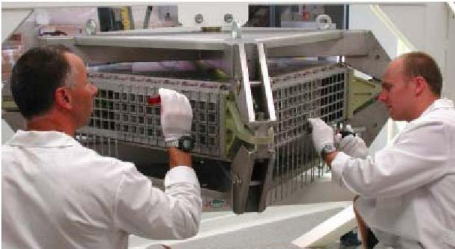
**Figure 15:** ECAL mechanical support structure
