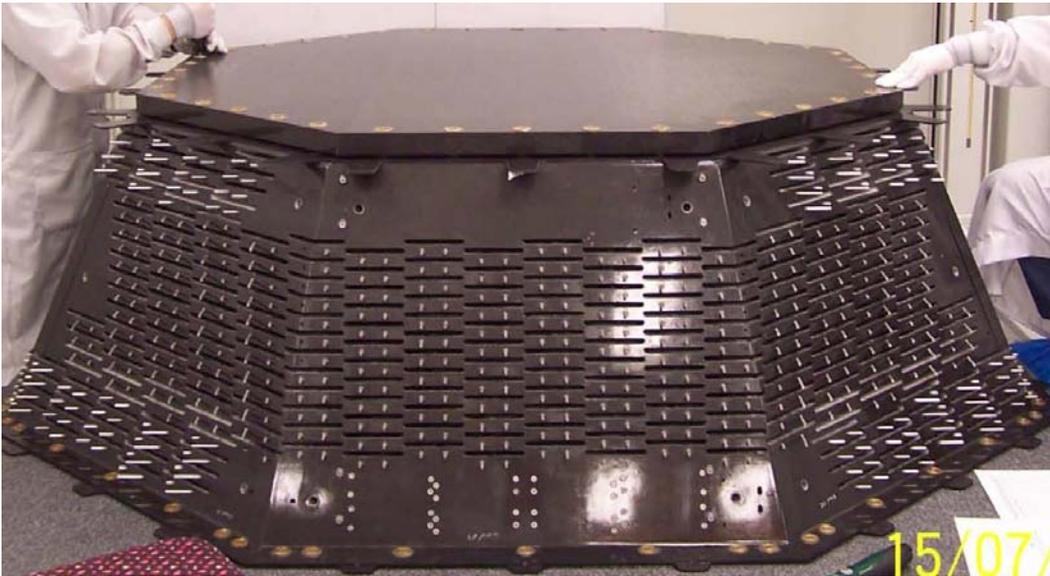
**Figure 5.** The TRD Octagon Support Structure
