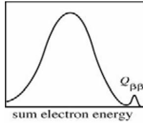
**Figure 9.** Sum energy spectrum, schematically, for  $2\nu 2\beta$  and  $0\nu 2\beta$  decays
