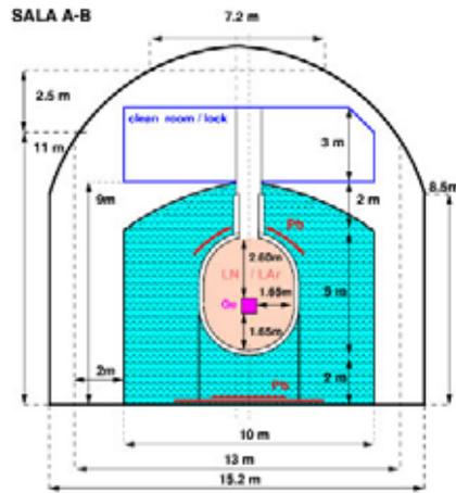
**Figure 13.** Schematic cross-section of the GERDA structures
