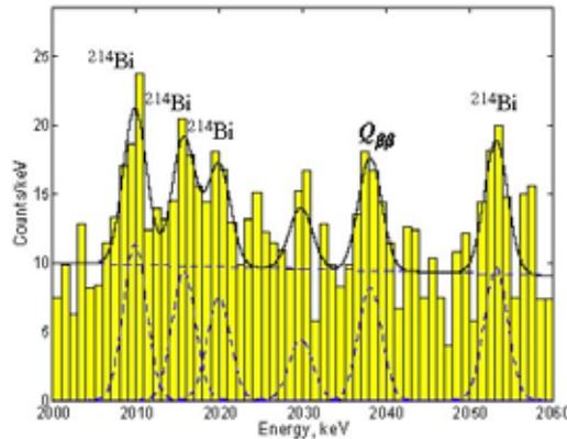
**Figure 10.** Sum energy spectrum from ref [31]. The labels identified the peaks as interpreted in ref [31]
