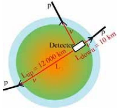
Figure 4. Principle of the MONOLITH proposal
