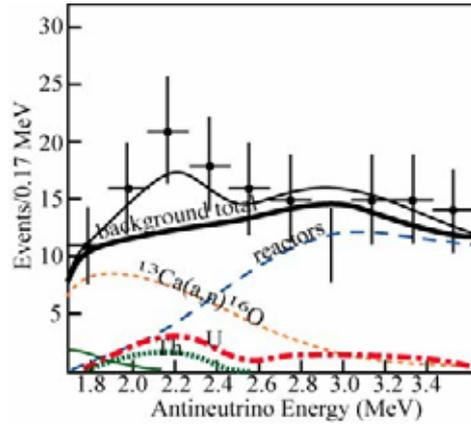
**Figure 14.** Electron antineutrino spectrum from KamLAND. Shown are the two principal backgrounds, the expected U and Th neutrino spectra and the total spectrum with these expectations
