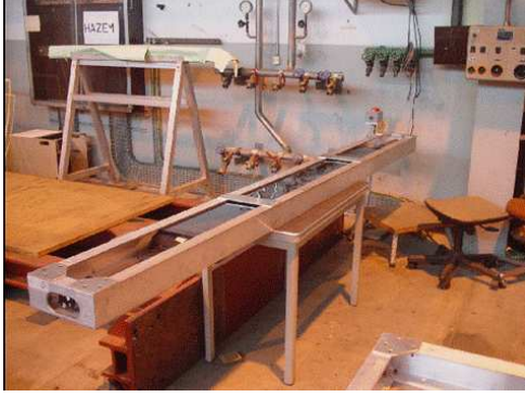
Figure 2. ACORDE module. This scintillator counter module consists of two superimposed scintillator counters with their corresponding photomultipliers active faces looking back to back. The active area is 188 \times 20 \text{ cm}^2 .
