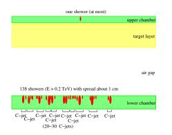
**Figure 1.** Illustration of the characteristics of Centauro-I. Two-storey chamber consists of the upper chamber, the target layer, air gap and the lower chamber. No (or one at least) shower is observed in the upper chamber but many (20 - 30) C-jets are observed in the lower chamber.
