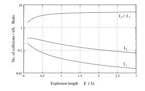
Figure 3. Expected number (divided by nN) of collisions in the upper chamber,  $I_1$ , and that in the target layer,  $I_2$ , when N small strangelets enter the chamber and explode into n nucleons respectively with explosion length L. The ratio between  $I_2$  and  $I_1$  is shown together. One can see that the number ratio increases gradually with increasing explosion length L.
