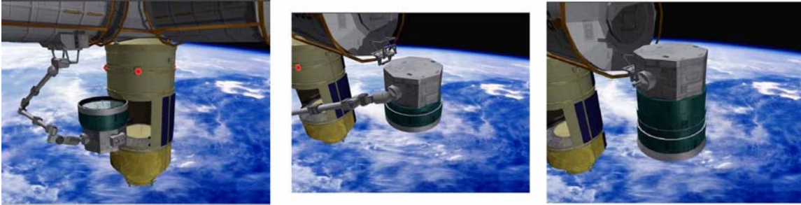
Fig. 1 Deployment of EUSO at the CEPF on ISS, transported by HTV unmanned transportation vehicle.
