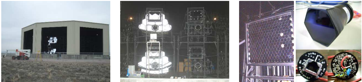
Figure 1. FD station (left), mirror (middle), PMT camera with pre-amplifier (right) for fluorescence measurement.
