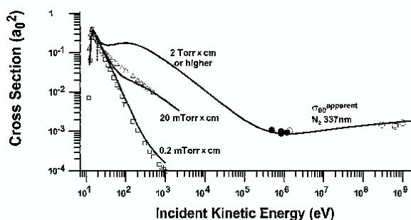
**Figure 2.** Apparent optical cross section  $\sigma_{00}^{ap}$  for 2P system of  $N_2$  versus electron energy as predicted by the model of ref. [6] for several  $NR$  values (continuous lines). Data deduced from measurements of Nagano et al. (●) and Kakimoto et al. (○) at high pressure are in good agreement with the model. This model also accounts for experimental results at low pressure ( $\Delta$ ,  $\square$ ). See [6] for more details.
