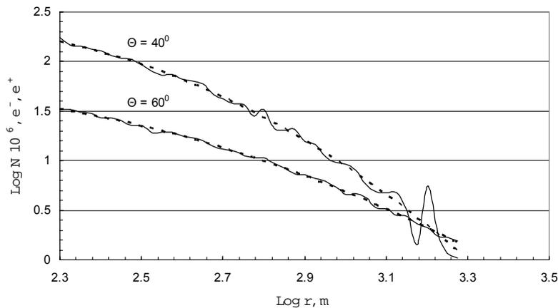
**Figure 1.** AIRES simulation of a gamma EAS of energy 100 EeV reaching the ground at a zenith angle of 40, 60 degrees, respectively. Dashed lines represent a polynomial fit suggested by Billoir et al [6].
