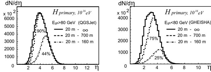
**Figure 3.** Distributions of muon pseudorapidities for different collecting distances for two ranges of grandmother hadron energies:  $E_{gh} > 80$  GeV (left) and  $E_{gh} < 80$  GeV (right)
